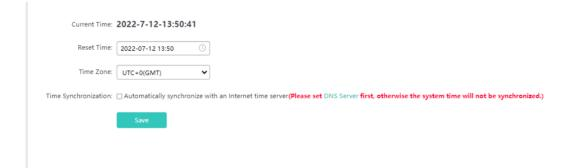
The page displays the current system time. You can set the system time manually or select **Automatically synchronize with** an **Internet time server**.
